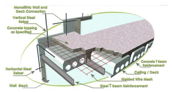
Figure (1) slab element
