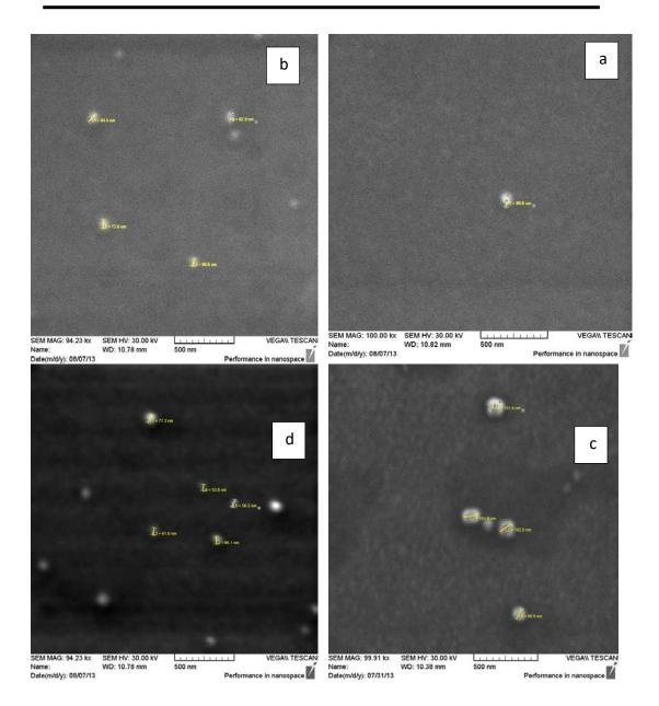
Figure (3) SEM image of Ag NPs prepared at 1.06 µm laser wavelength and different laser energy (a-100, b-200 and c-600 d-800) m J and 100 pulse.
