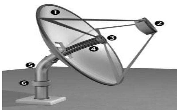
Figure (1) shows solar lighting system, where 1 is primary reflector, 2 is secondary reflector, 3 is fiber mount, 4 is large core optical fiber, 5 is angled
