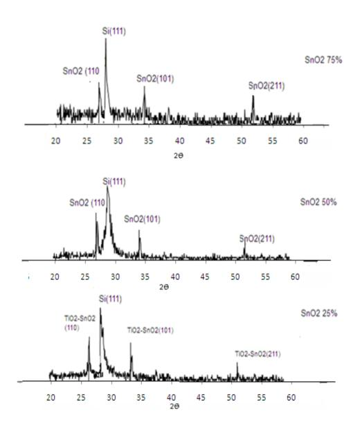
Figure (2) XRD patterns of (TiO<sub>2</sub> -SnO<sub>2</sub>) films grown on Si
