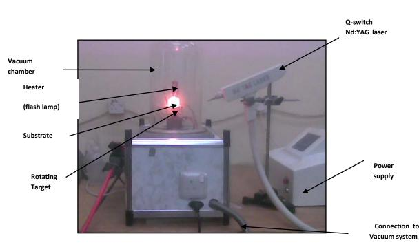
Figure (I) Experimental setup
