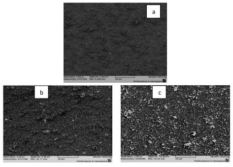
Figure (3) SEM images of (TiO<sub>2</sub> -SnO<sub>2</sub>) films grown on Si at different SnO<sub>2</sub> content%a) 25% b) 50% c) 75.
