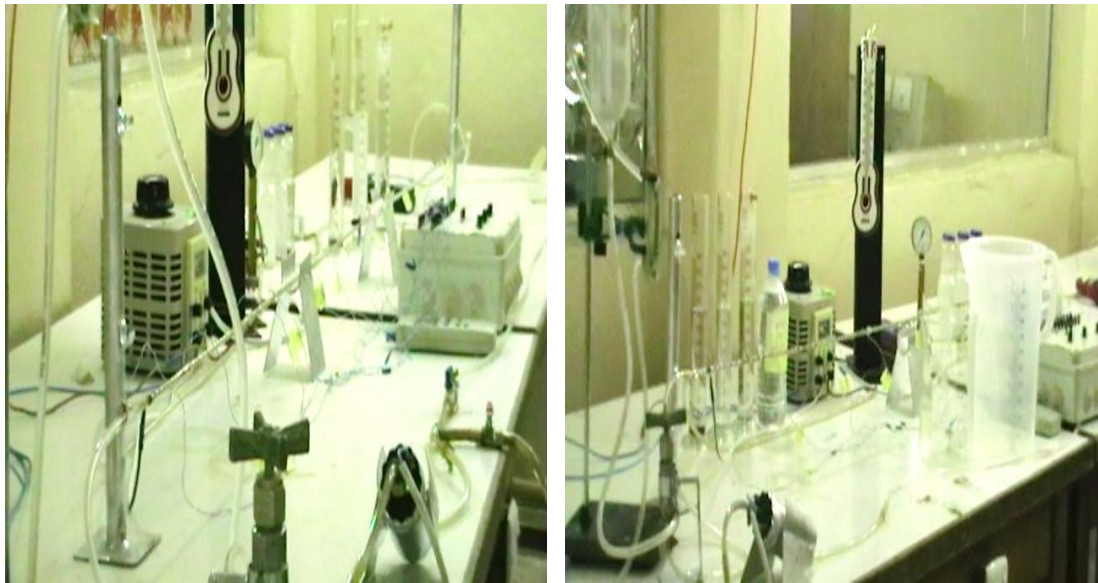
Figure (2) The experimental system of the convective heat transfer and flow characteristics for nanofluid, [33].
