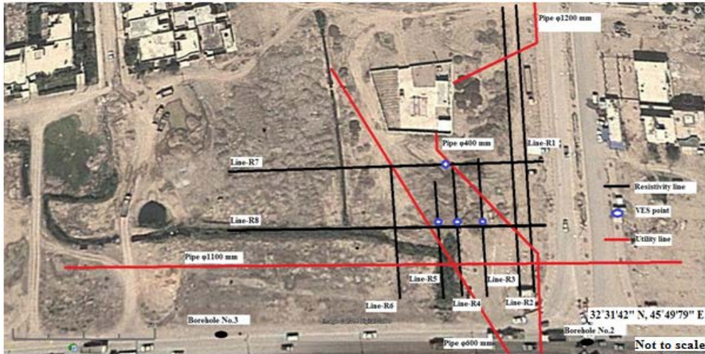
Figure (4) Acquisition geometry for 2D resistivity in site.
