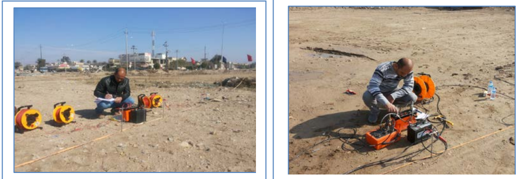
(a) (b) Plate(2) ABEM Terrameter SAS 4000 with accessories for: (a) 1D and (b) 2D configurations.
