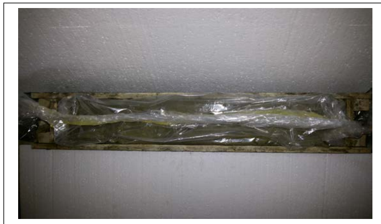
Figure (3) Airtight envelop around concrete specimen
