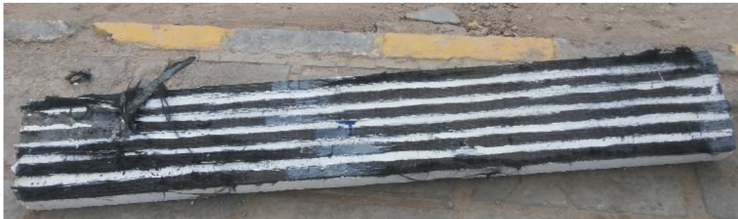
Figure(8.3) Cracks pattern after failure for slab SHS2
