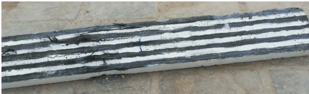
Figure (8.2) Cracks pattern after failure for slab SHS1
