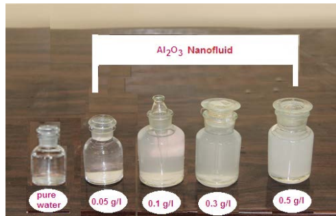
Figure (6) Photographs of the water-Al 2 O 3 nanofluids preparation
