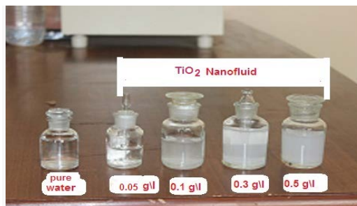
Figure (7) Photographs of the water-TiO 2 nanofluids preparation
