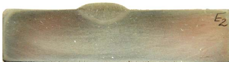
e. I=400 amp, V=29 v, S=8.3 mm/s, P=2.62 mm, W=11.85 mm, HAZ w =1.36 mm
