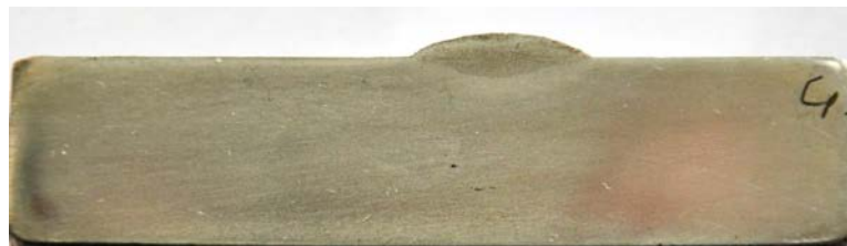
b. I=280 amp, V=26 v, S=3.3 mm/s, P=1.45 mm, W=10.98 mm, HAZ w =1.31 mm
