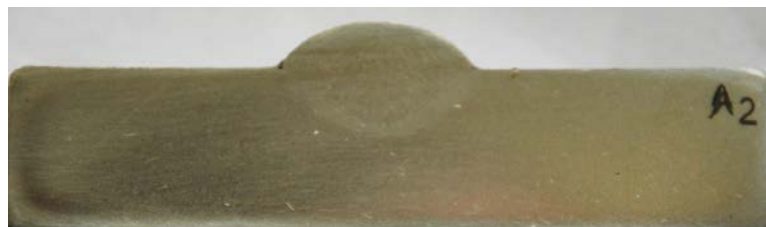
f. I=460 amp, V=29 v, S=6.6 mm/s, P=4.21 mm, W=12.40 mm, HAZ w =1.46 mm
