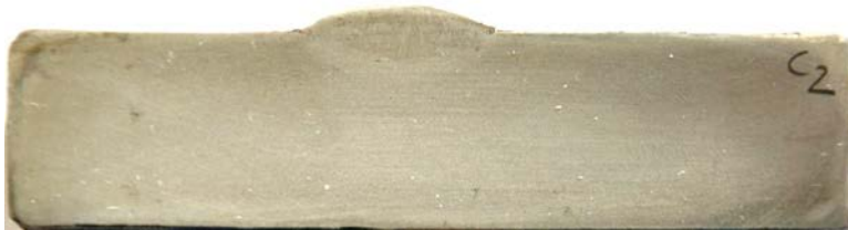
c. I=280 amp, V=29 v, S=5 mm/s, P=2.03 mm, W=11.58 mm , HAZ w =1.23 mm
