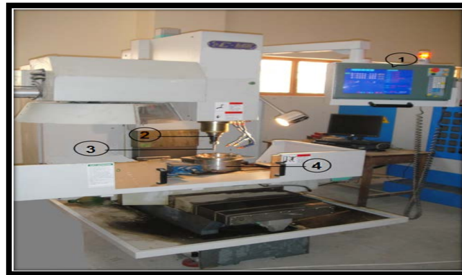
Figure (2): CNC milling machine used in the experimental campaign (1) machine controller, (2) tool holder, (3) forming tool, (4) forming frame.
