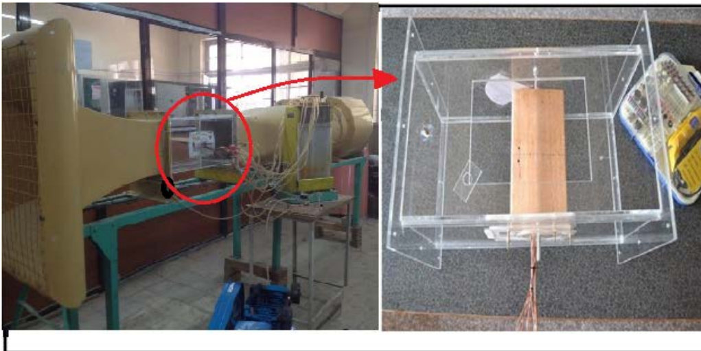
Figure(8). Subsonic wind tunnel and the test section.
