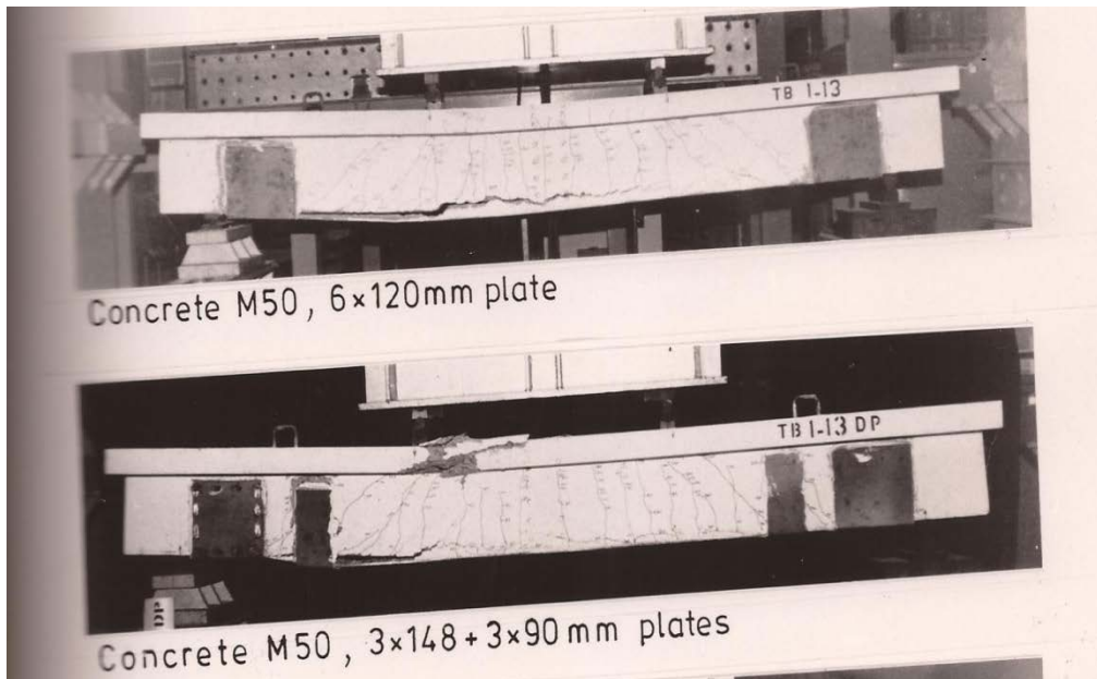
Figure(5): Typical Debond Failure of Plated Beams
