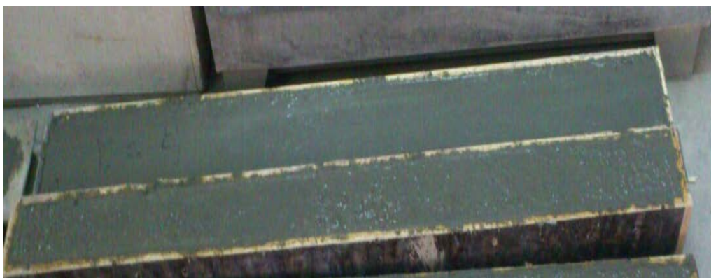
Plate (4)Unbonded Beam Casting
