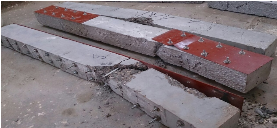
Plate (7)Failure Mode by Yielding of Steel Platefor UnbondedTechnique
