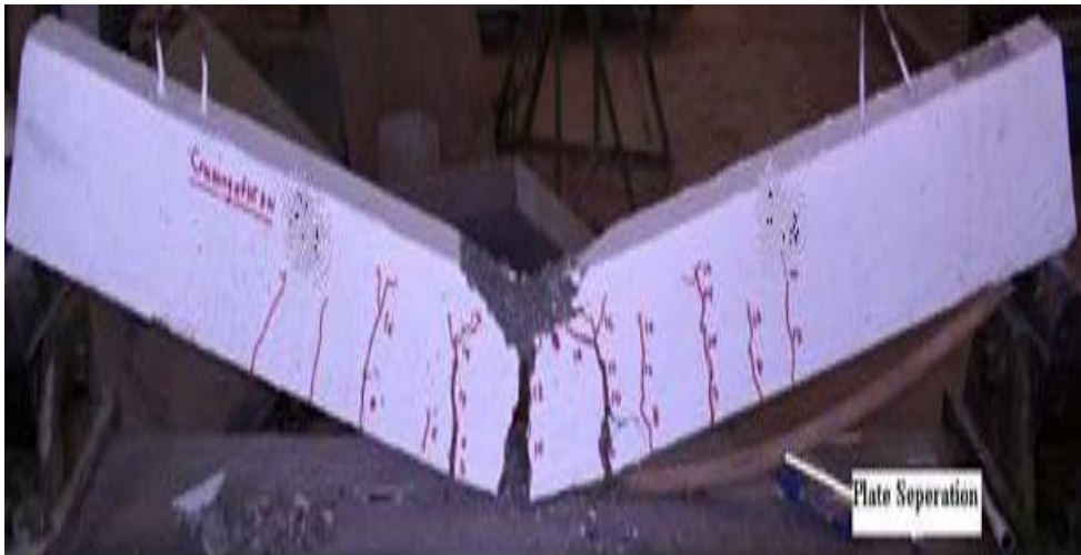
Plate (5) Failure Mode by Separating Steel Plate
