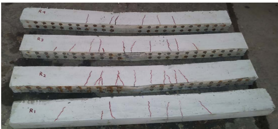
Plate (6) Failure Mode by Yielding of Steel Plate for bonded Technique
