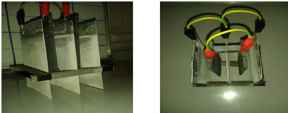
Figure (2) photography of two graphite electrodes as anode, and three commercial
