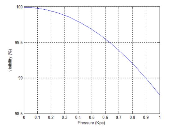
Fig. (9): The effect pressure on the visibility of MZIM (248 K) (0 - 40 Kpa)
