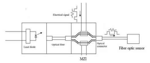
Fig. (2): Illustration visibility of a MZIM with fiber optic sensor to monitoring environmental
