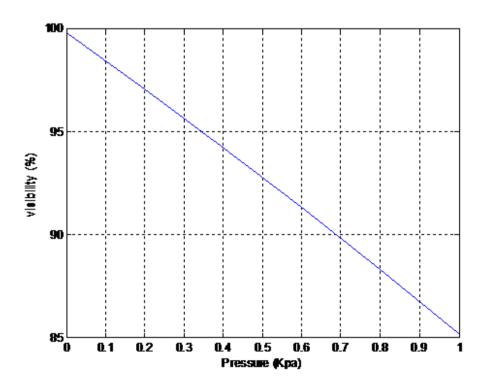
Fig. (10): The effect pressure on the visibility of MZIM (223 K) (0 - 40 Kpa)
