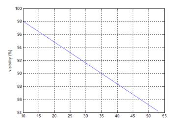
Fig. (6): The effect strain on the visibility of MZIM (258 K) (10 - 55  $\mu\epsilon$ )
