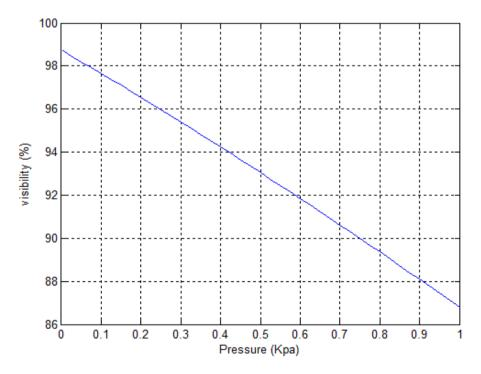
Fig. (8): The effect pressure on the visibility of MZIM (293 K) (0 - 40 Kpa)
