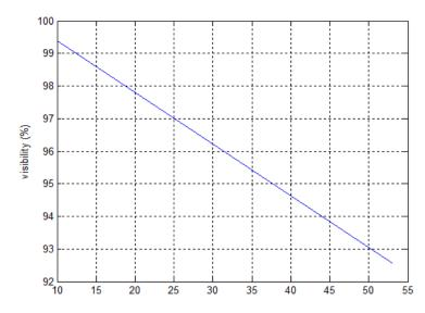
Fig. (4): The effect strain on the visibility of MZIM (333 K) (10 - 55  $\mu\epsilon$ )
