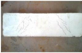
**Figure 9h.** A700R (Group A, potable water, heating at 500°C, rapid cooling)
