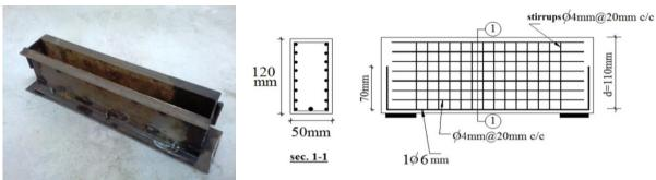
Figure 1. Typical steel mold
