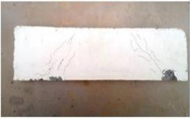
**Figure 9f.***A500R* (Group A, potable water, heating at 500°C, rapid cooling)
