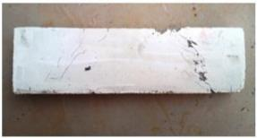
**Figure 11d.** *BCR-III* (*Group B, potable water, cycling heating 350°C, 650°C and 850°C, gradual cooling*)
