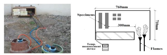
Figure 4.The used steel furnace with heating resources and specimens
