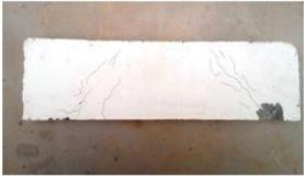
**Figure 9d.** A300R (Group A, potable water, heating at 300°C, rapid cooling)
