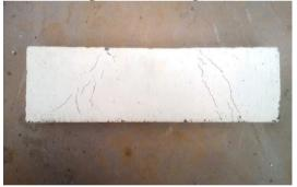
**Figure 9e.**A500G (Group A, potable water, heating at 500°C, gradual cooling)
