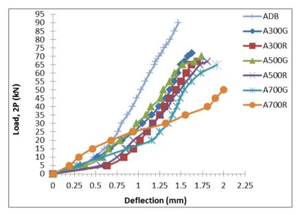
Figure (8): Load-Deflection for the beams of group A, measured at mid-span
