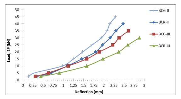
Figure 10. Load-Deflection for the beams of Group B, measured at mid-span
