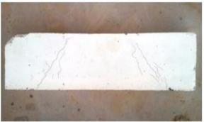
**Figure 9g.** A700G (Group A, potable water, heating at 700°C, gradual cooling)
