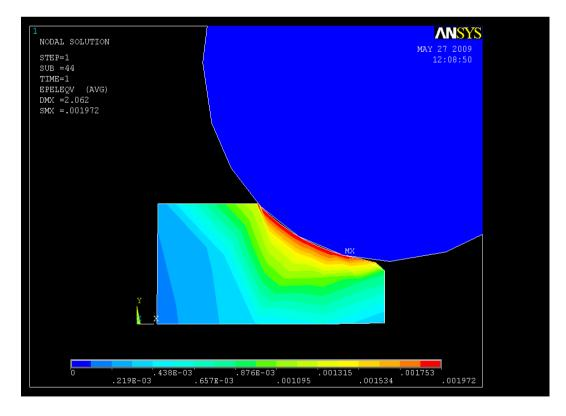
Figure (4): Nodal Elastic Strain Distribution when Rolling Pressure =300Mpa and  $\mu_f$ =0.3
