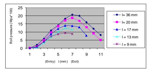
Figure (8): Calculated Distribution of Roll Pressure for Various Stage of Rolling of Aluminum at Entry and Exit
