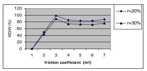
Figure (10): The effect of friction coefficient on the ratio of plastic energy Dissipation to the total energy
