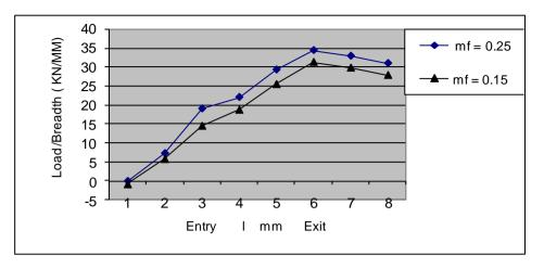
Figure (9): Variation of Calculated Load with advancement of Aluminum Strip when  $\mu_f$ =0.15, 0.25 at Entry and Exit
