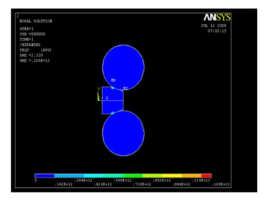
Figure (7): Shape Change of Front End of an Aluminum Strip according to Loading Step and Rolling Pressure.
