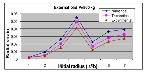
**Figure (13):** Distributions of radial strain on initial radius when the external load equal 800 kg comparison of theory result, F.E.M and Experimental.
