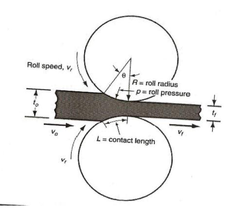
Figure (1): General idea of Modeling of Plane – Strain Rolling
