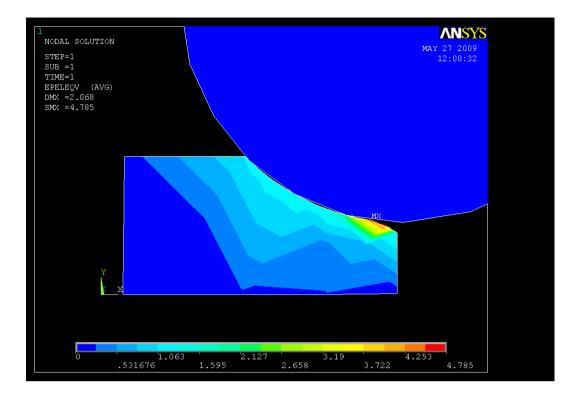
Figure (5): X-Displacement (flow direction) with Rolling Pressure =300 Map,  $\mu_f$ =0.3 and Reduction of Area = 40%
