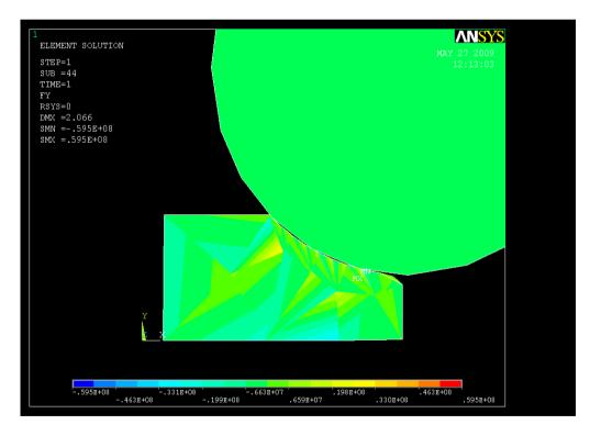
Figure (6): Shear Force in y-direction when Reduction of Area =30% Rolling Pressure equal to 300 Mpa and  $\mu_f$ =0.3
