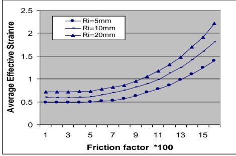
**Figure (11):** The Average Effective Strain with different Contact Surfaces Between Aluminum and Rollers with Variation Friction Factor
