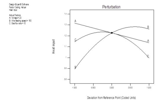
Fig. (11): Perturbation of Heat Input on Wire Feeding Speed and Gas Flow Rate.
