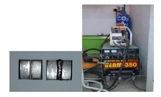
Fig. (1): CO<sub>2</sub>-MAG Welding Machine and Specimens Before and After Welding.
