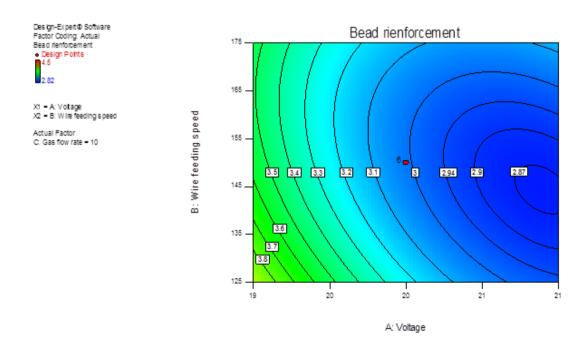
Fig. (8): Contour Graph of Bead Reinforcement as A functions of Voltage and Wire Feeding Speed at 10 L/min Gas Flow Rate.
