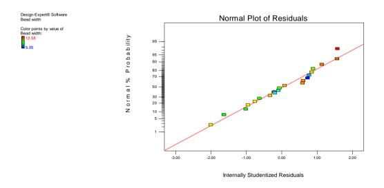
Fig. (3): Normal Probability Plot of Residuals for Bead Width Data.
