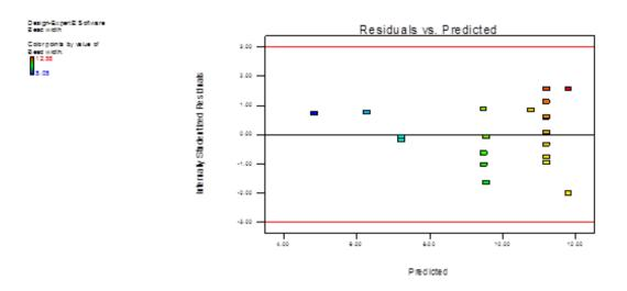
Fig. (4): Residual versus Predicted Responses for Bead Width Data.
