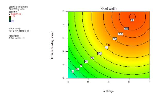
**Fig. (7):** Contour Graph of Bead Width as A functions of Voltage and Wire Feeding Speed at 10 L/min Gas Flow Rate.
