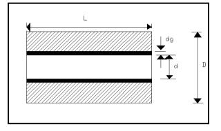
**Fig. (1):** Schematic diagram of work piece and layer of the abrasive media (L=40mm, D=45mm, d=19 mm).
