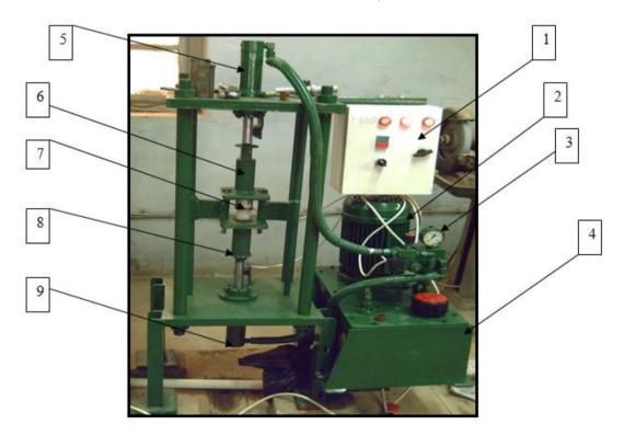
**Figure (2):** AFM setup :(1) control box, (2)electrical pump, (3) pressure gage, (4) hydraulic unit, (5) upper hydraulic cylinder, (6) upper media cylinder, (7) workpiece and fixture,(8) lower media cylinder, (9)lower hydraulic cylinder
