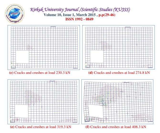
Figure.(16): Cracks and concrete crushes patterns at deep beam strengthened by horizontal CFRP sheet of 0.7 mm thickness at different load stages.
