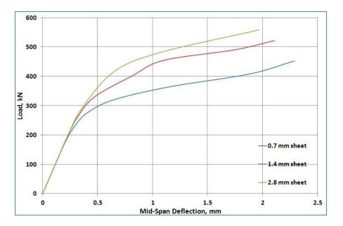
Figure.(14): Load-deflection curves for deep beams strengthened with horizontal CFRP sheet.
