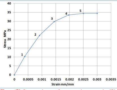
Figure.(50: Stress-strain curve for concrete in compression [2]
