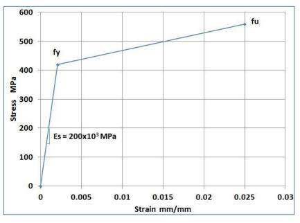
Figure.(6): Stress-strain curve for steel bars
