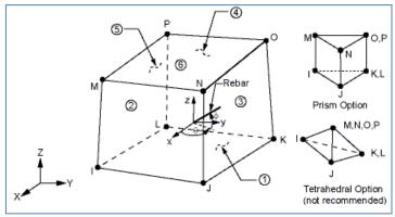
Figure.(1): Concrete element SOLID65 geometry [12]
