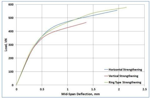
Figure.(12): Load-deflection curves for deep beams strengthened with 2.8 mm CFRP sheet.
