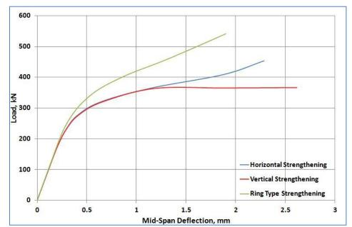
Figure.(10): Load-deflection curves for deep beams strengthened with 0.7 mm CFRP sheet.
