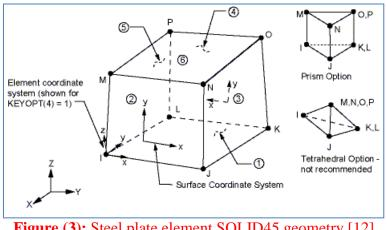
Figure.(3): Steel plate element SOLID45 geometry [12]
