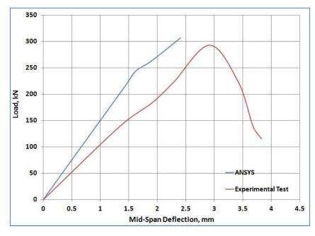
Figure.(9): Load-deflection curves for deep beams with large opening tested by Dipti [1] and simulated by ANSYS
