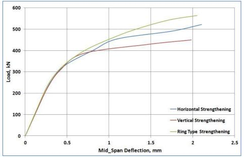
Figure.(11): Load-deflection curves for deep beams strengthened with 1.4 mm CFRP sheet.
