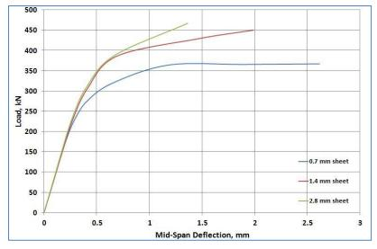
Figure.(13): Load-deflection curves for deep beams strengthened with vertical CFRP sheet
