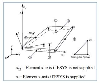
Figure.(4): CFRP laminates element SHELL41 geometry [12]
