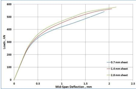
Figure.(15): Load-deflection curves for deep beams strengthened with ring type CFRP sheet.
