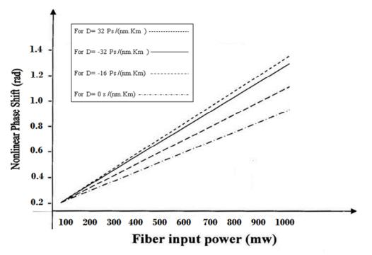
Fig. 2 Effect of fiber input power on nonlinearity.
