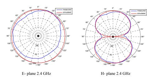
(8-a) Simulated and measured results at 2.4 GHz
