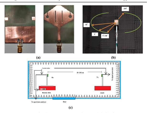
(a). Printed antenna (b). Antenna in an anechoic chamber (c). Diagram for the Tx. & Rx antenna in the chamber Fig. (7) Practical antenna through measurement
