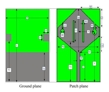
Fig. (2) the final proposed antenna
