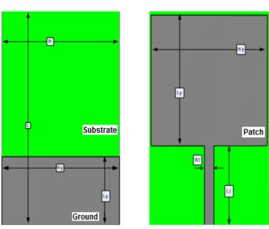
Ground plane Patch plane Fig. (1) the conventional proposed antenna
