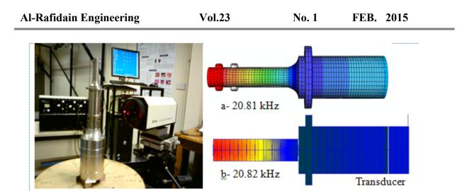
Figure 10 Comparison of (a) FE predicted and (b) EMA measured longitudinal mode and modal frequency
