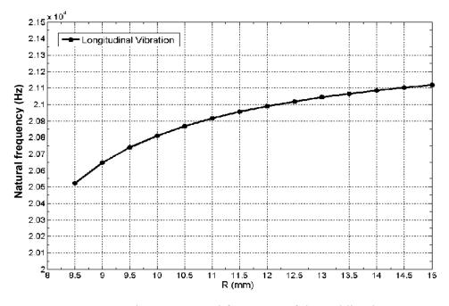
Figure 7 Natural frequency of the welding horn
