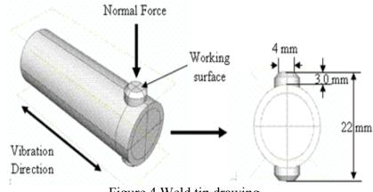
Figure 4 Weld tip drawing
