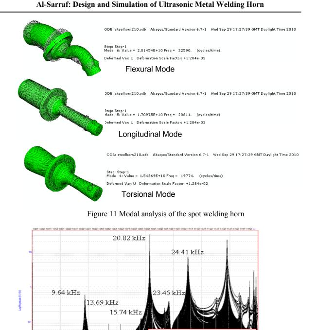
Figure 12 Modal analysis spectrum and vibration mode of welding horn
