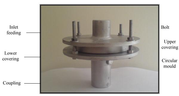
Figure (4): Photograph of the assembly of mould.
