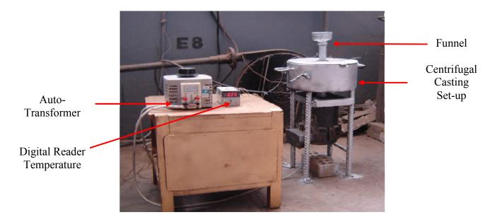
Figure (2): Photograph of centrifugal casting apparatus.
