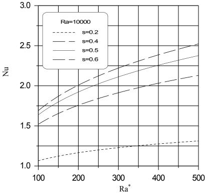
Figure (5) shows the effect of Ra\* on the Nu for different dimensionless heat source length ( $\hat{s}=0.2, 0.4, 0.5$  and 0.6) and Ra=10<sup>4</sup>
