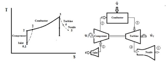
Figure (1) Brayton Cycle for Jet propulsion [7]
