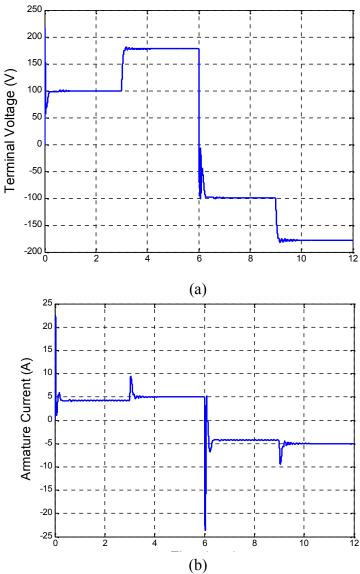
4. Figure (6) Average terminal voltage and armature current responses of the separately excited DC motor in the forward and reverse motoring modes.
