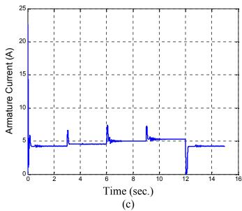
1. Figure (3) (a) speed (b) average terminal output voltage and (c) armature current responses of the separately excited DC motor in the forward motoring mode.
