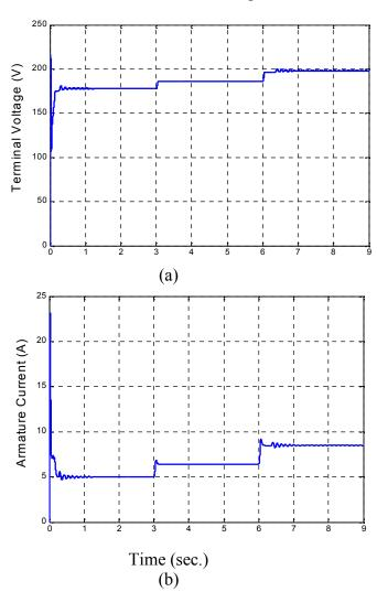
Figure (8) (a) average terminal output voltage and (b) armature current responses of the DC machine with variable load torque in the forward motoring mode.
