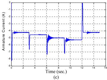
2. Figure (4) (a) speed (b) average terminal output voltage and (c) armature current responses of the separately excited DC motor in the reverse motoring mode.
