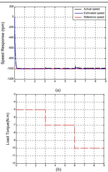
7. Figure (9) Speed response of the separately excited DC machine with variable load torque in the reverse motoring mode.
