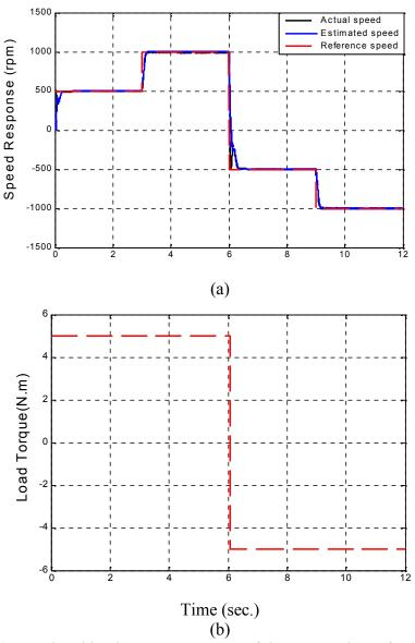
3. Figure (5) Speed and load torque responses of the separately excited DC motor in the forward and reverse motoring modes.
