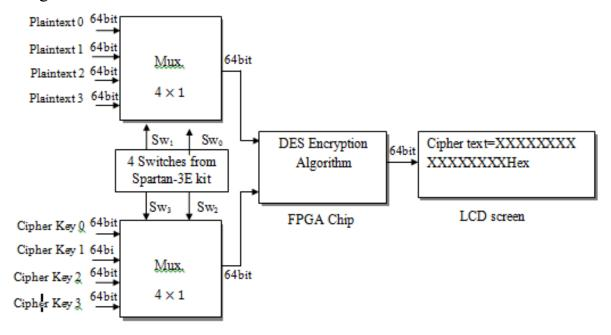
Fig. 6 A hardware implementation for input/output unit for the DES Encryption algorithm.
