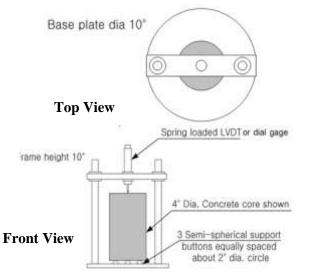
Figure (2) Schematic of a Measuring Frame (AASHTO TP 60 2004) [15]
