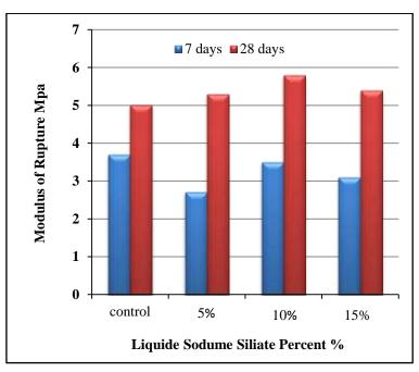
Figure (5) : Effect of liquid Sodium Silicate percent on modulus of rupture
