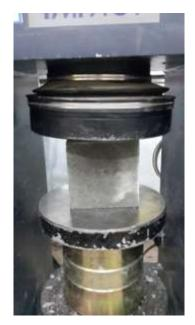
Plate (1) : Compressive strength apparatus
