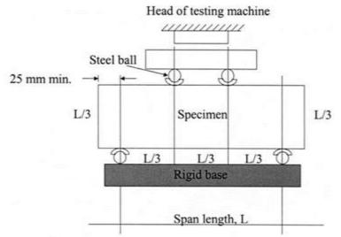
Figure (1) : Test for modulus of rupture
