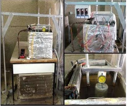
Plate (3): CTE measuring apparatus
