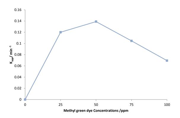
Figure 3: Pseudo-first order rate constant at varying dye concentration. Conductions: semiconductor dosage 700 mg/200 mL, pH= 5.4, temperature 278.15  $^{\circ}$ K, UV light intensity 6 x10<sup>-5</sup> ensien.s<sup>-1</sup>.
