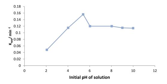
Figure5:Pseudo-first order rate constant at varying initial pH.Conductions:dye conc.50ppm, semiconductor dosage 700 mg/200 mL,temperature 278.15 °K, UV light intensity 6 x10<sup>-5</sup> ensien.s<sup>-1</sup>.
