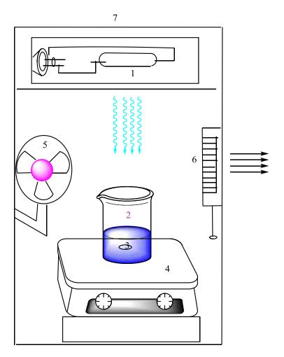
Scheme 1: Schematic Diagram of Experimental Set-up. Where: High pressure mercury lamp(400 W)(1), 400 cm<sup>3</sup> Pyrex glass beaker (2), Teflon bar (3), magnetic stirrer (4), fan (5), pump fan (6) and wooden box (7).
