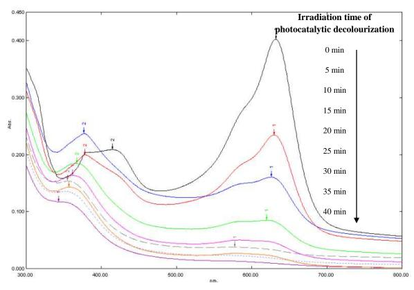
Figure 2: UV-Visible absorption spectra change at different time intervals.
