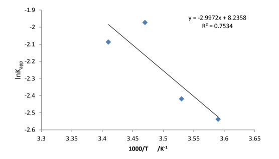
Figure 6: Pseudo-first order rate constant at varying temperature. Conductions: dye conc. 50 ppm, semiconductor dosage 700 mg/200 mL, pH= 5.4, temperature 278.15-293.15  $^{\circ}$ K, UV light intensity 6 x10<sup>-5</sup> ensien.s<sup>-1</sup>.
