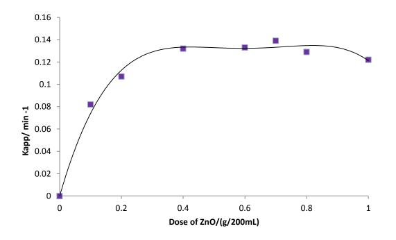
Figure 4: Pseudo-first order rate constant at varying semiconductor dosages. Conductions: dye conc. 50 ppm, pH= 5.4, temperature 278.15  $^{\circ}$ K, UV light intensity 6 x10<sup>-5</sup> ensien.s<sup>-1</sup>.
