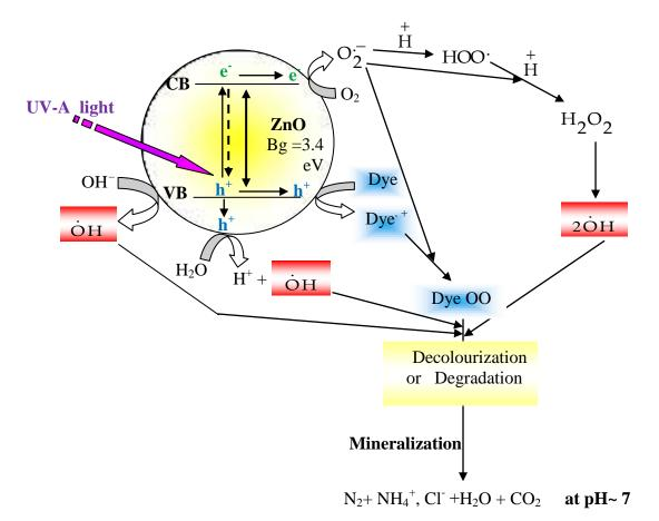
Scheme 2:Schamitic diagram for more accepted mechanism (Dye/semiconductor/ UV light system)(modified from reference [25]).
