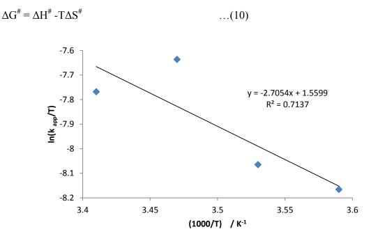
Figure 7: Eyring plot of  $(\ln(K_{app}/T))$  vs.1/T. Conductions: dye conc. 50 ppm, semiconductor dosage 700 mg/200 mL, pH= 5.4, temperature 278.15-293.15 °K, UV light intensity 6 x10<sup>-5</sup> ensien.s<sup>-1</sup>.
