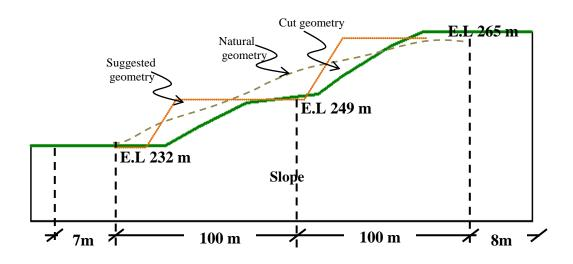
Figure. (4): Schematic Diagram of Natural, Cut, Suggested geometries
