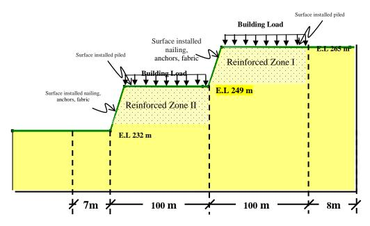
Figure. (2): Schematic Diagram of Suggested Geometry Slope
